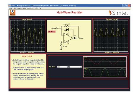
Though we are leaving in digital world, Analog Electronics is a vital part of electronics engineering; for understanding advance technologies in electronics, the student have to have the knowledge of basic principles of Electronics. And for this we came with very good software "Simtel Analog Electronics", which comprises of simulations, animations, along with mandatory theory to understand fundamental concepts of Analog Electronics.
